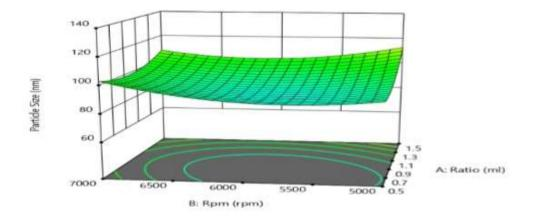
Three Dimensional Response surface plot for particle size
